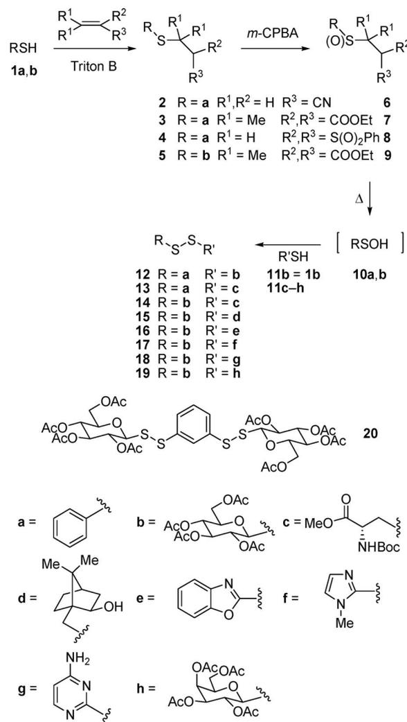
Scheme 1. Synthesis of unsymmetrical disulfides **12–20**.
