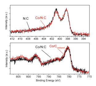
**Figure 2.** X-ray photoelectron spectra of N 1s orbital in Co/N:C and pristine N:C (top), and Co-3/2 p orbital on Co/N:C and Co/C $_{undoped}$  (bottom). The metal loadings for both Co/N:C and Co/C $_{undoped}$  are 1.3 mmol g $^{-1}$ .
