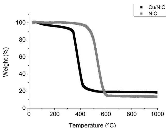
**Figure S4.** Thermal gravimetric analysis (TGA) curves of Cu/N:C and plain N:C. TGA showed the mass loss of N:C at 500°C, whereas the Cu/N:C has a mass loss at a lower temperature. This difference indicates that the copper oxidises the nitrogen-doped surface during the treatment, thereby lowering the temperature of the mass loss. The difference in weight percentage at the end of the measurement around 600 °C is the copper oxide that is present in the Cu/N:C sample.
