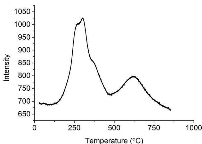
**Figure S2.** Temperature programmed reduction (TPR) spectrum for Cu/N:C. The temperature programmed reduction (TPR) shows multiple copper oxide species presence inside the copper oxide catalyst. At 300 °C copper oxide is reduced, where multiple peaks indicate multiple copper oxide species. At 600 °C the support N:C is reduced. <sup>[1]</sup>
