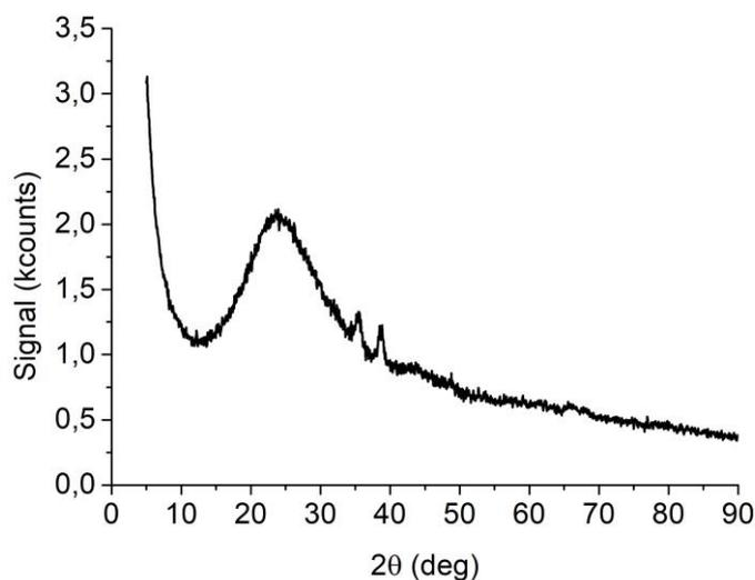
**Figure S3.** X-ray powder diffraction (XRD) spectrum for Cu/N:C. X-ray diffraction showed a broad peak at 25° which is typical for carbon. The small peaks at 36.1° (-111) and at 39° (111) are typical for CuO.<sup>[2]</sup>
