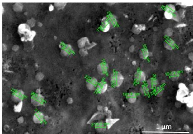
**Figure S1.** Scanning electron micrographs of Cu/N:C. The size of the copper oxide is ca. 200-250 nm. Scanning electron microscopy (SEM) of Cu/N:C catalyst with particle measurements. The average size of the copper oxide spherical particles is ca. 200-250 nm. Furthermore, the clusters are evenly distributed onto the support surface.
