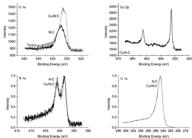
**Figure 2.** XPS spectra of the Cu/N:C and pristine N:C samples showing the oxygen 1s, Cu 1/2p and 3/2p, nitrogen 1s and carbon 1s binding energies. Impregnation of copper oxide on the N:C increases the oxygen content but does not affect the nitrogen or carbon peaks. Note that the nitrogen and carbon graphs are normalised for clarity.
