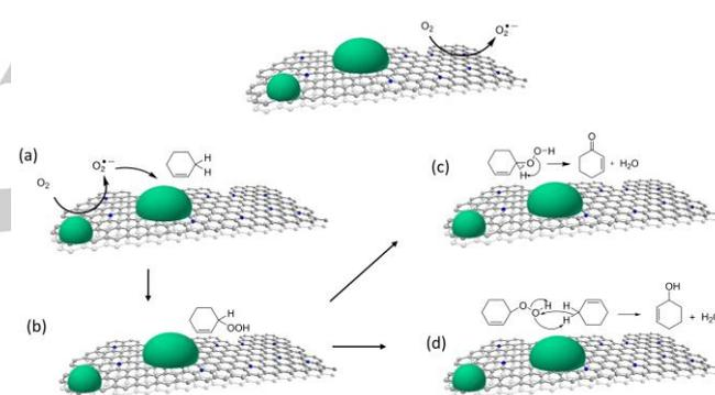
**Figure 3.** Proposed reaction pathways for the catalytic oxidation of cyclohexene with molecular oxygen in the presence of Cu/N:C. (a) Oxygen activation at the support surface followed by radical migration into solution. (b) Insertion of activated oxygen into the allylic C–H bond to give the adsorbed hydroperoxide **D** followed by either (c) rearrangement to the ketone **A** and water or (d) reaction with another cyclohexene molecule to give two molecules of the alcohol **C**.
