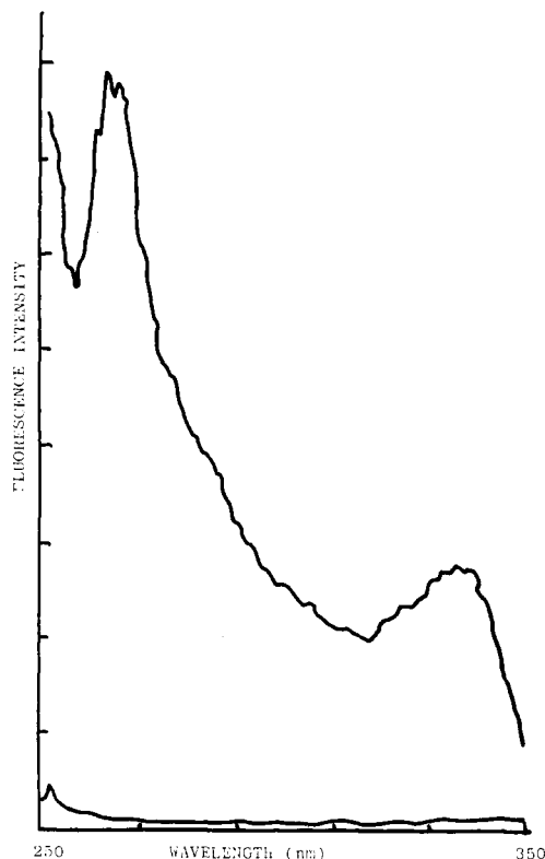
Figure 6. Fluorescence spectra of assemblies with and without surfactant pyrene as dopant: (—) S_{16A} :arachidate 1:1 (---) Py_{16A} :arachidate 1:1, ( \cdots ) S_{16A} :arachidate 1:1 with 4% Py_{16A} .
