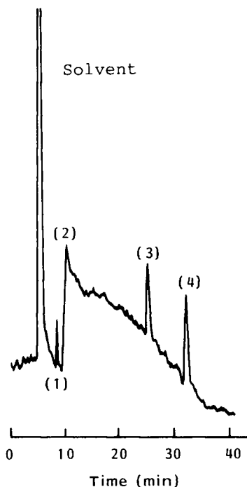
Figure 2—Liquid chromatogram of partially hydrolyzed products of G_2 - \beta -CyD. Key: (1) glucose; (2) maltose; (3) G_1 - \beta -CyD; (4) G_2 - \beta -CyD. The increase in the baseline at \sim 11 min was due to the elution of salts such as KCl and NaCl.
