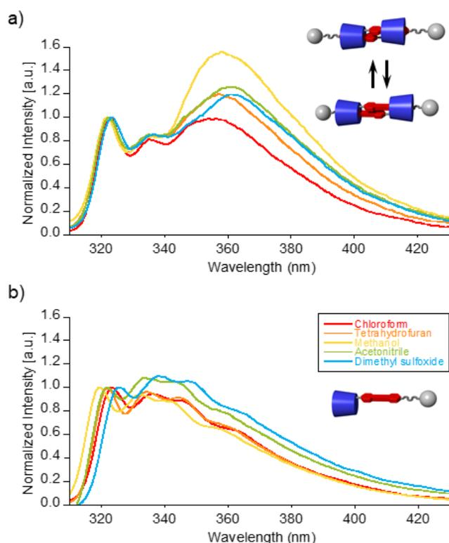
**Figure 2.** Fluorescence spectra of (a) rotaxane **2** and (b) stoppered monomer **3**. Conditions: [**2**] =  $2.6 \times 10^{-7}$  M, [**3**] =  $1.9 \times 10^{-6}$  M, excitation at the maximum absorption wavelength in the range of 311–316 nm.
