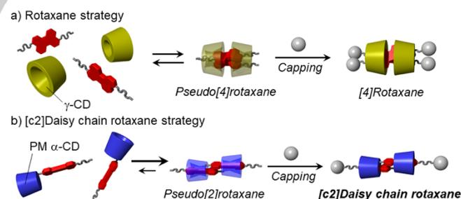
**Figure 1.** Synthetic strategies for rotaxanes insulating two  $\pi$ -conjugated molecular cores.
