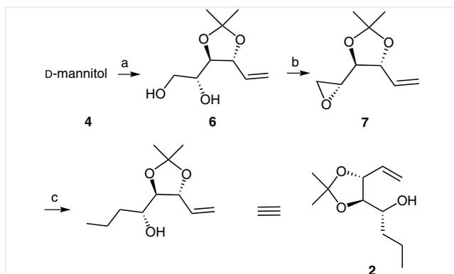
**Scheme 2** Synthesis of the alcohol fragment **2**. Reagents and conditions: (a) ref. 7; (b) (i)  $\text{Bu}_2\text{SnO}$ ,  $\text{TsCl}$ ,  $\text{Et}_3\text{N}$ ,  $\text{CH}_2\text{Cl}_2$ , r.t., 30 min; (ii)  $\text{K}_2\text{CO}_3$ ,  $\text{MeOH}$ , r.t., 1 h, 75%; (c)  $\text{EtMgBr}$ ,  $\text{CuI}$ ,  $-20^\circ\text{C}$  to r.t., 84%.
