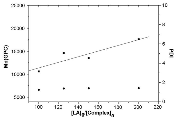
Fig. 6. Polymerization of L-LA catalyzed by 2 in THF at 60 °C. The relationship between Mn (■) ((PDI (●)) of the polymer and the initial mole ratio  $[LA]_0/[Complex]_0$  is shown.
