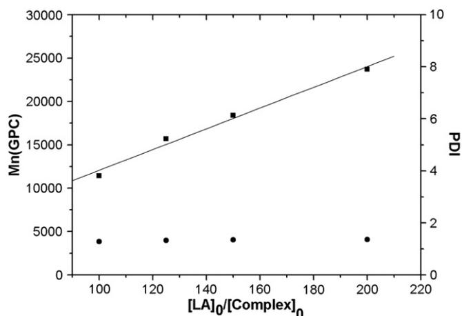
**Fig. 3.** Polymerization of L-LA catalyzed by 1 in THF at 60 °C. The relationship between Mn (■) ((PDI (●)) of the polymer and the initial mole ratio  $[\text{LA}]_0/[\text{Complex}]_0$  is shown.
