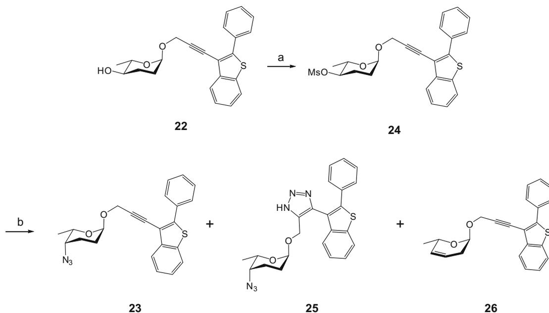
**Scheme 2.** Reagents and conditions: (a) MsCl, Et<sub>3</sub>N, 0 °C, 99%; (b) NaN<sub>3</sub>, DMF, 120 °C, 40% for **23**, 30% for **25**, 19% for **26**.
