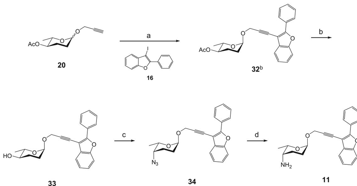
**Scheme 4.** Reagents and conditions: (a) 5% Pd(PPh<sub>3</sub>)<sub>2</sub>Cl<sub>2</sub>, 10% CuI, piperidine, 73%; (b) K<sub>2</sub>CO<sub>3</sub>, methanol, 99%; (c) PPh<sub>3</sub>, DPPA, DIAD, -20 °C → rt, 83%; (d) PPh<sub>3</sub>, H<sub>2</sub>O 91%. <sup>b</sup> The pure β anomers were isolated, and the subsequent transformations were performed separately, see Section 2.2.3.
