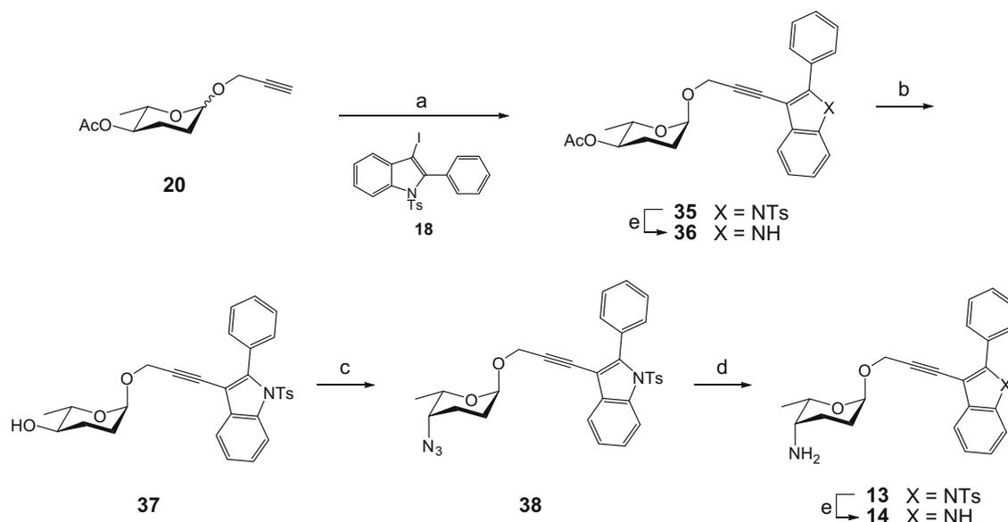
**Scheme 5.** Reagents and conditions: (a) 5% Pd(PPh<sub>3</sub>)<sub>2</sub>Cl<sub>2</sub>, 10% CuI, piperidine, 51%; (b) K<sub>2</sub>CO<sub>3</sub>, methanol, 89%; (c) PPh<sub>3</sub>, DPPA, DIAD, -20 °C → rt, 73%; (d) PPh<sub>3</sub>, H<sub>2</sub>O 86%; (e) *n*-Bu<sub>4</sub>NF, THF, rt, 61% for **36** and 75% for **14**. <sup>b</sup> The pure β anomers were isolated, and the subsequent transformations were performed separately see Section 2.2.3.
