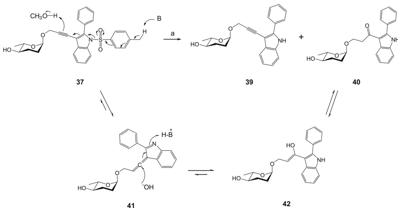
**Scheme 6.** Reagents and conditions: (a) KOH, CH<sub>3</sub>OH, reflux, 65% for **40**.
