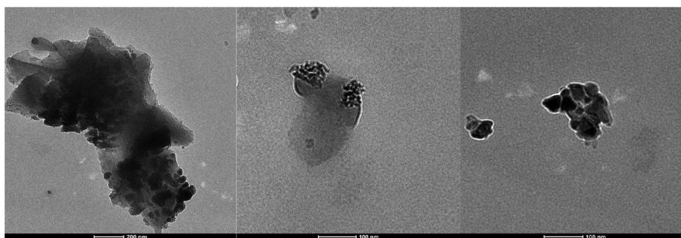
Fig. 6 TEM images of the  $\text{Al}_2\text{O}_3/\text{CuI}/\text{PANI}$  nanocatalyst.
