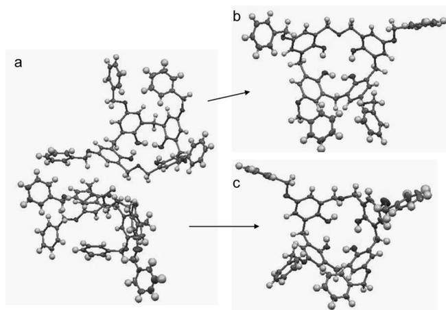
Figure 3. Solid-state structure of **6**: (a) orientations of the two independent molecules in the unit cell; (b) and (c) different views of the molecules, highlighting the orientations of the CH<sub>2</sub>OCH<sub>2</sub> bridge.
