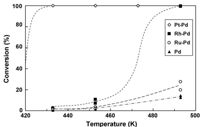
**Fig. 5.** Oxidation of benzene over noble-metal-loaded Pd membranes (O<sub>2</sub>: 10 ml/min, O<sub>2</sub>:benzene = 1:0.125).
