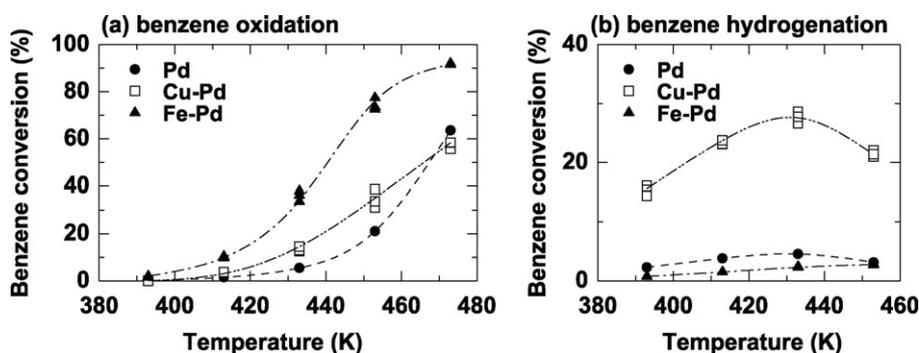
**Fig. 7.** Related reactions over transition-metal-loaded Pd membranes: (a) oxidation of benzene (O<sub>2</sub>: 2 ml/min, O<sub>2</sub>:benzene = 1:0.026) and (b) hydrogenation of benzene by permeated hydrogen (H<sub>2</sub>: 10 ml/min, H<sub>2</sub>:benzene = 5:0.026).
