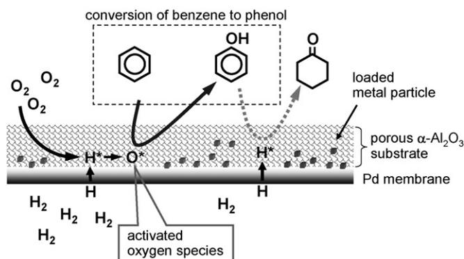
**Fig. 1.** Schematic illustration of one-step conversion of benzene to phenol and consecutive hydrogenation over metal-loaded Pd membrane reactor.
