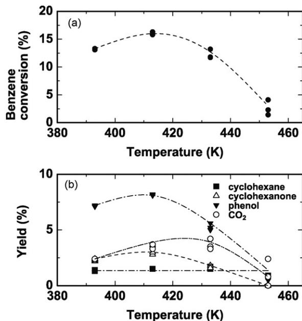
**Fig. 6.** Effect of reaction temperature on hydroxylation of benzene over Cu–Pd membrane: (a) conversion and (b) yield.
