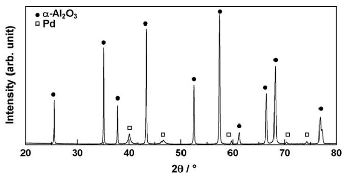
Fig. 3. XRD pattern of Pd-loaded  $\alpha$ -Al<sub>2</sub>O<sub>3</sub> tube before CVD treatment.
