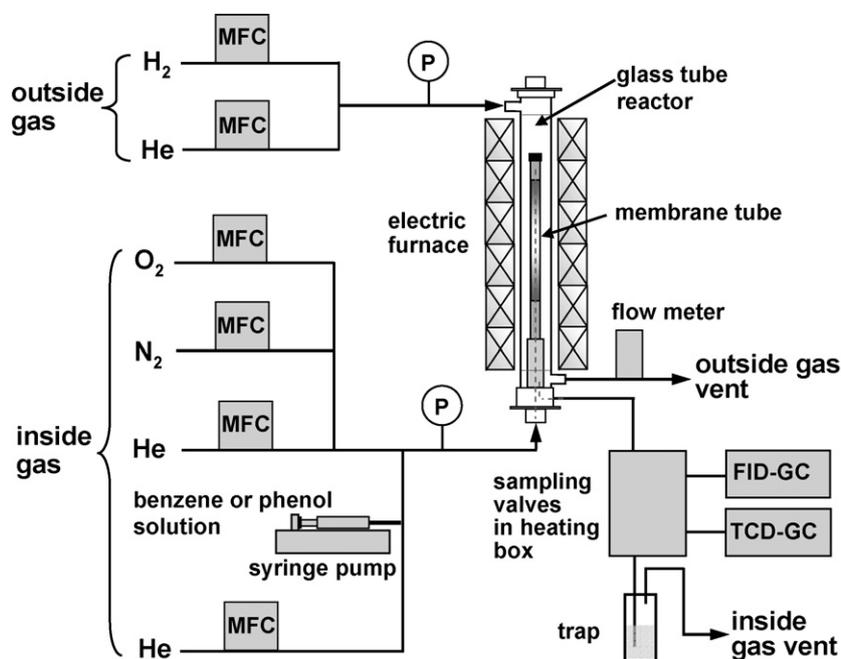
Fig. 2. Diagram of Pd based membrane reactor.
