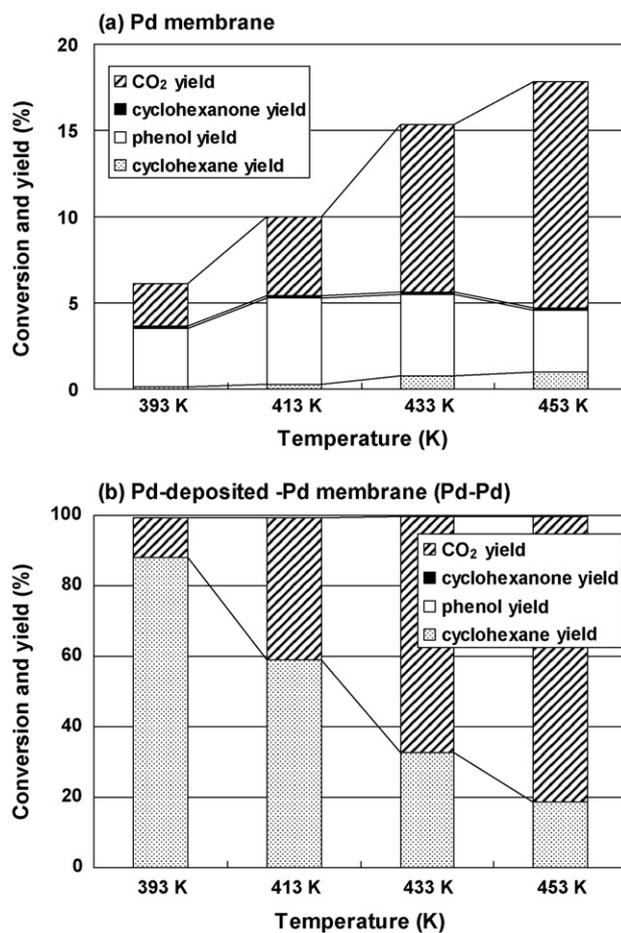
Fig. 4. Effect of reaction temperature on hydroxylation of benzene over (a) Pd membrane and (b) Pd-deposited Pd membrane (Pd–Pd).
