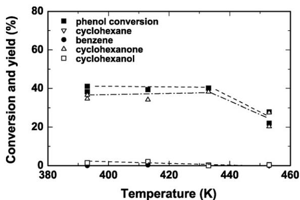
Fig. 8. Reaction of phenol and permeated hydrogen over length of 3 cm on Pd membrane ( $H_2$ : 10 ml/min, 1 wt.% phenol aqueous solution: 0.2 ml/min).
