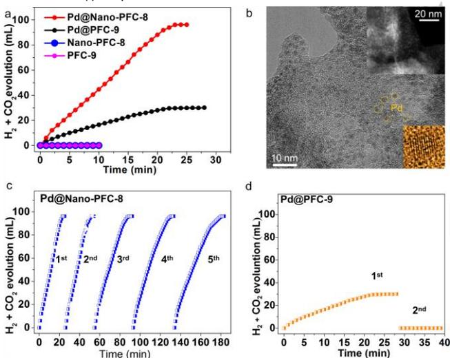
**Figure 4.** (a) Gas evolution with Pd@Nano-PFC-8 and Pd@PFC-9 catalysts. (b) TEM images of Pd@Nano-PFC-8 after five recycling runs. Insets show the dark-field TEM image (top) and HRTEM image (down). The recyclability of (c) Pd@Nano-PFC-8 and (d) Pd@PFC-9 for FA dehydrogenation. Pd contents are 1.20 wt% for Pd@Nano-PFC-8 and 0.70 wt% for Pd@PFC-according to the inductively coupled plasma analyses.
