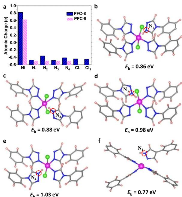
**Figure 2.** (a) Bader charge analyses for the Ni(II) center and the coordinated nitrogen, chlorine in PFC-8 and PFC-9. Computational optimized configurations and binding energies of a proton with the ligands in PFC-8 (b-e) and PFC-9 (f).
