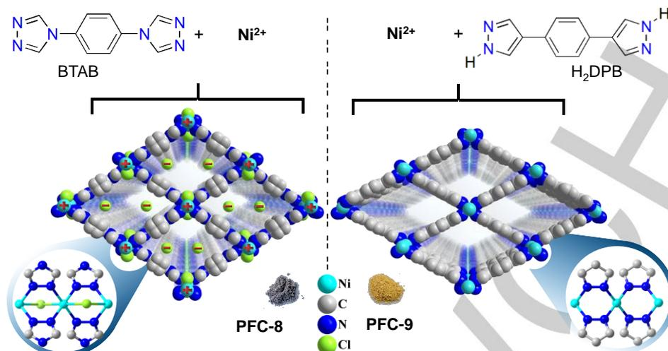
Scheme 1. Schematic representation of the structures of cationic PFC-8 and neutral PFC-9
