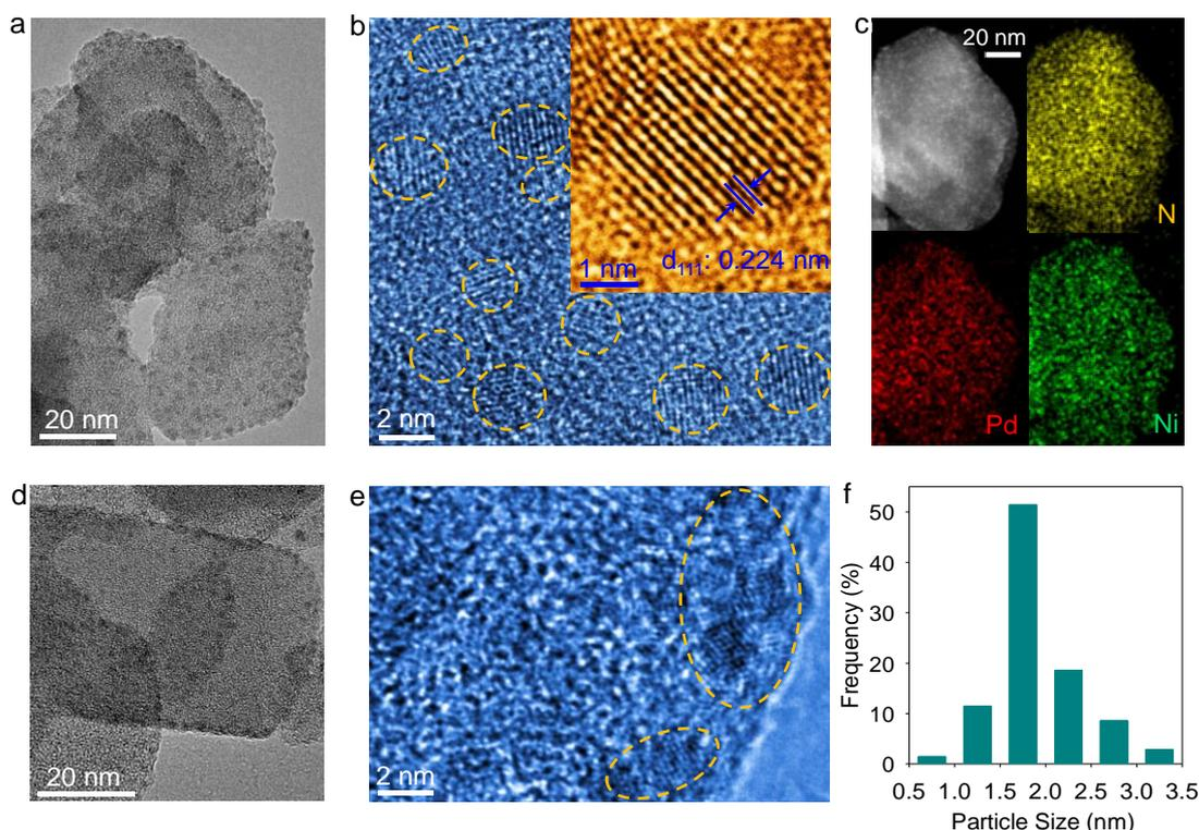
**Figure 3.** (a, b) HRTEM images and (c) Dark-field TEM-EDX mapping of Pd@Nano-PFC-8, Pd NPs are circled in yellow. (d, e) HRTEM images of Pd@PFC-9. (f) Pd particle size distribution in Pd@Nano-PFC-8.
