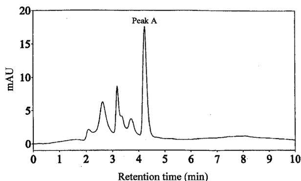
**Fig. 4.** HPLC Chromatogram of the Reaction Mixture of Collected Fraction D and the XTT Solution.
