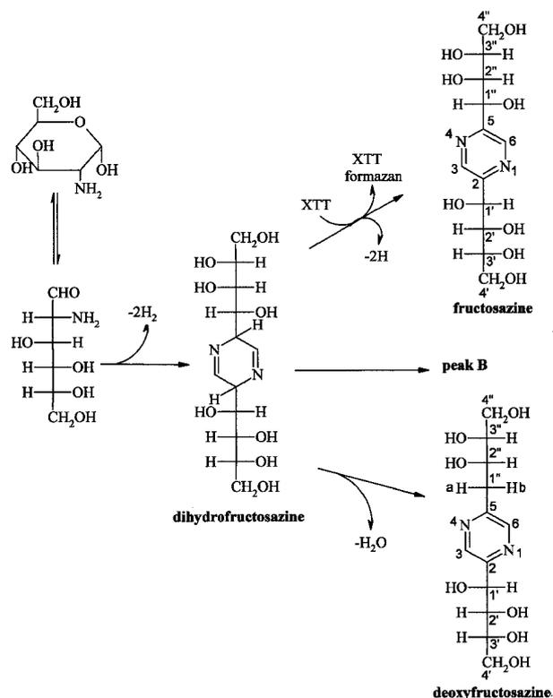
Fig. 5. Reduction Mechanism for XTT by D-Glucosamine Derivatives.
