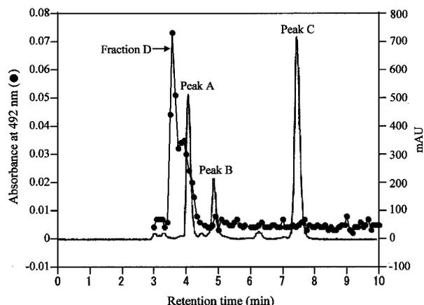
**Fig. 1.** HPLC Chromatogram of the D-Glucosamine Derivatives and XTT Reducibility of the Fractionated Eluate (● absorbance at 492 nm).
