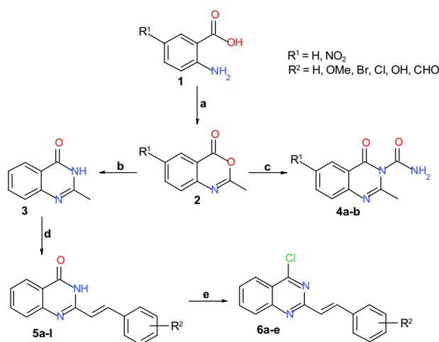
Scheme 1. Synthesis of the studied compounds: (a)  $\text{Ac}_2\text{O}$  MW; (b)  $\text{NH}_3\text{aq}$  MW; (c) urea; (d) aldehyde MW; (e)  $\text{POCl}_3$ .
