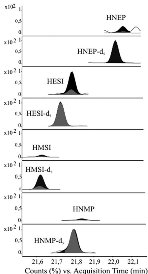
**Figure 3.** Chromatogram of a native urine sample from a person representing the general population not occupationally exposed to NMP and NEP (quantifier and qualifier are in black and gray). The concentrations of 5-HNMP, 2-HMSI, 5-HNEP, and 2-HESI are 129, 87, 143, and 235  $\mu\text{g/L}$ , respectively.
