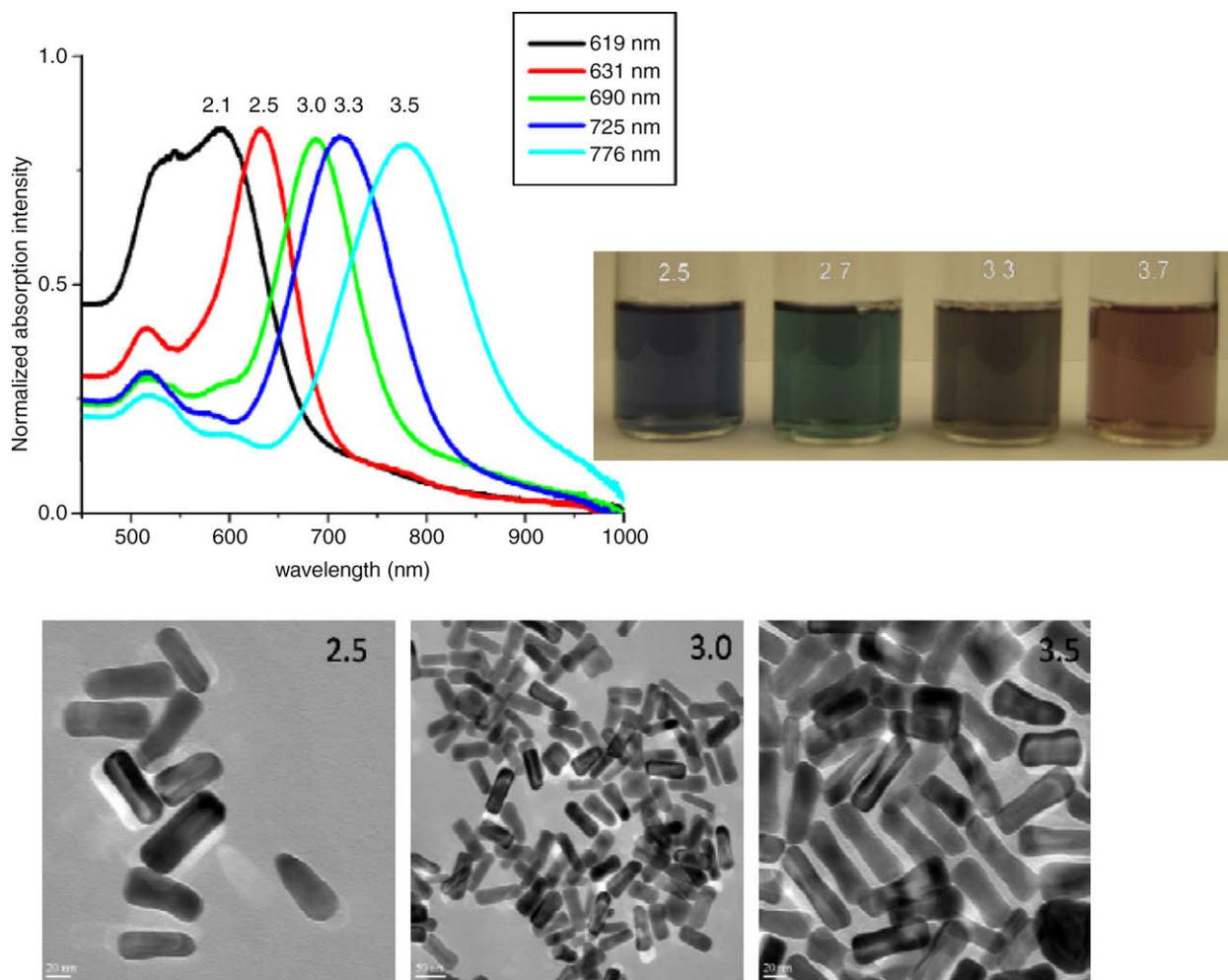
Fig. 1. Absorption spectra, photograph and TEM images of gold nanorods of different aspect ratios.
