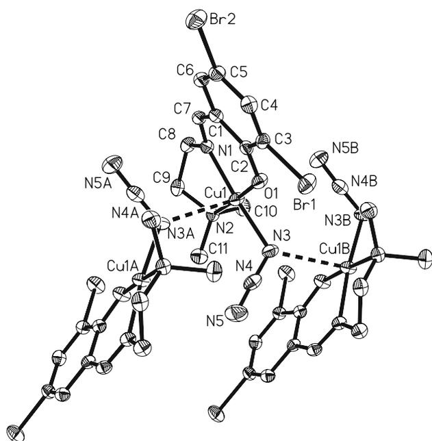
**Fig. 2** Molecular structure of  $[\text{Cu}(\text{L2})(\mu_{1,1}\text{-N}_3)]_n$  at 30% probability ellipsoids. Atoms labeled with the suffix A and B are at the symmetry positions  $-1/2 + x, 1/2 - y, 1 - z$  and  $1/2 + x, 1/2 - y, 1 - z$ , respectively. H atoms have been omitted for clarity
