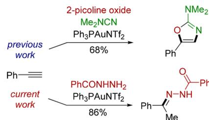
benzohydrazide reacted smoothly with phenylacetylene in the presence of  $\text{Ph}_3\text{PAuNTf}_2$  to yield the appropriate acylhydrazone, whereas pyridine *N*-oxides did not participate in the observed transformation.
