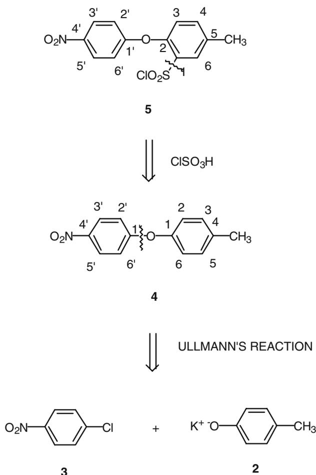
**Fig. 1** Retrosynthetic analysis. Structures of compounds 2–5
