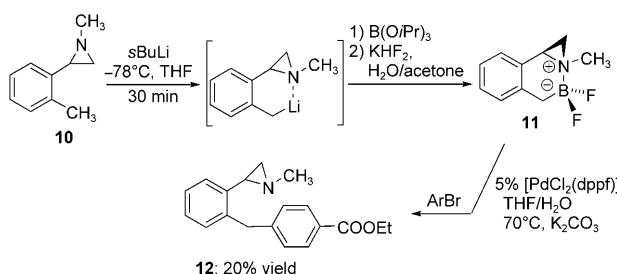
Scheme 4. Synthesis and reaction of difluoroborate **11**.
