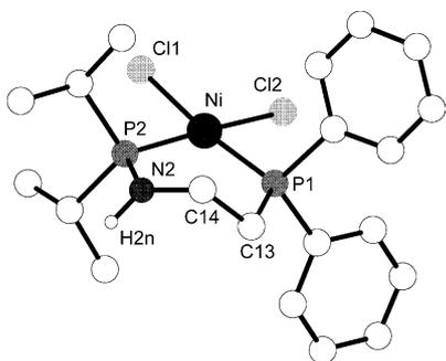
Fig. 1. X-ray structure of  $\text{NiCl}_2(\text{PH}_2\text{PCH}_2\text{CH}_2\text{NHPPri}_2)$  (**8**). Selected bond lengths (Å) and angles ( $^\circ$ ) Ni–P(1) 2.173(2), Ni–P(2) 2.186(2), Ni–Cl(1) 2.196(2), Ni–Cl(2) 2.226(2), P(1)–C(13) 1.822(6), C(13)–C(14) 1.524(9), C(14)–N(2) 1.448(8), N(2)–P(2) 1.668(6); P(1)–Ni–P(2) 96.1(1), Cl(1)–Ni–Cl(2) 90.1(8), N(2)–P(2)–Ni 117.3(2), C(14)–Ni–P(2) 125.7(4).
