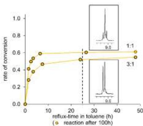
**Figure 3.** Rate of conversion of Kocheshkov reaction for different educt ratios of (2):(1), inlays:  $^1\text{H-NMR}$  spectra of  $\beta$ -hydrogen region after 25h
