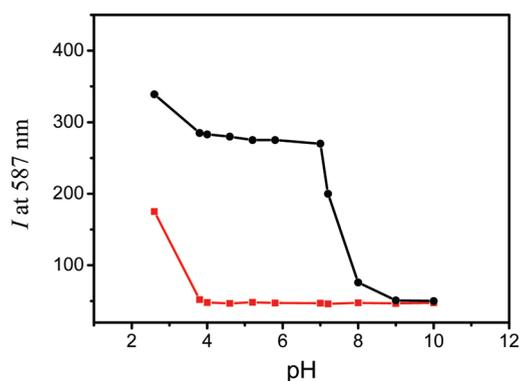
**Figure 5.** Variation of fluorescence intensity at 587 nm for the AD-SRhB/ $\beta$ -CD-DNS supramolecular-complex aqueous solution ( $1 \times 10^{-4}$  M) with and without  $\text{Fe}^{3+}$  ( $1 \times 10^{-4}$  M) as a function of pH ( $\lambda_{\text{exc}}$  410 nm; black curve, with  $\text{Fe}^{3+}$ ; red curve, without  $\text{Fe}^{3+}$ ).
