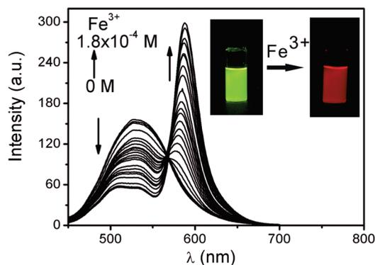
**Figure 2.** Fluorescence spectra ( $\lambda_{\text{exc}}$  410 nm) of the AD-SRhB/ $\beta$ -CD-DNS supramolecular-complex aqueous solution ( $1 \times 10^{-4}$  M) upon addition of ferric ion (pH 7.0). (Inset) Photographs of the supramolecular-complex aqueous solution before and after the addition of ferric ion ( $1.4 \times 10^{-4}$  M) under UV light irradiation.
