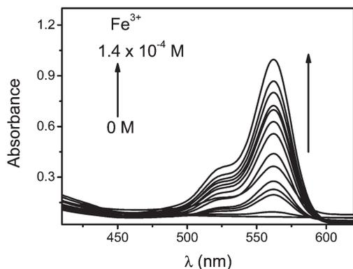
**Figure 1.** Absorption spectra of the AD-SRhB/ $\beta$ -CD-DNS supramolecular-complex aqueous solution upon addition of ferric ion (pH 7.0).
