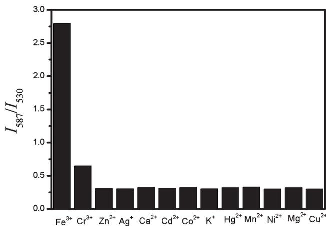
**Figure 3.** Fluorescence intensity changes ( $I_{587}/I_{530}$ ) of the AD-SRhB/ $\beta$ -CD-DNS supramolecular-complex aqueous solution ( $1 \times 10^{-4}$  M) upon addition of different metal ions ( $8 \times 10^{-5}$  M) ( $\lambda_{\text{exc}}$  410 nm, pH 7.0).
