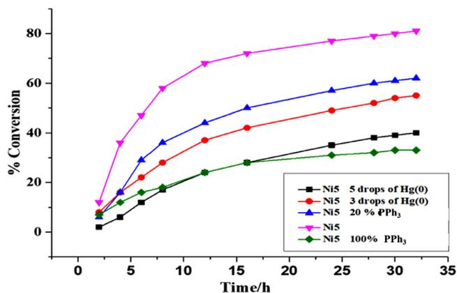
**Fig. 3.** The plot of conversion vs time in the showing TH of acetophenone using complex Ni5 in the presence of Hg(0) and phosphine poisoning agents.
