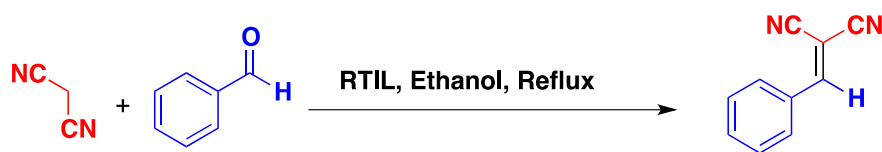
Scheme 3. Synthesis of \alpha -cyanoacrylates using RTILs
