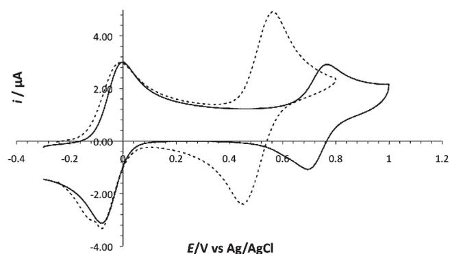
Figure 9. Cyclic voltammograms of 2 (dotted line) and 4 (solid line) in the presence of decamethylferrocene (dmfc, shown at ca.  $-0.04$  V vs Ag/AgCl) in DCM. Scan rate = 500 mV/s. For other experimental conditions, see Table 3 and the Supporting Information.
