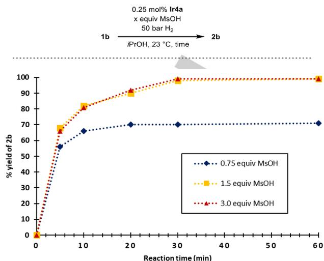
**Figure 2.** Influence of the acid concentration in the reaction rate. Conditions: 0.3 mmol **1a**, 0.23 / 0.45 / 0.90 mmol MsOH, 0.25 mol% **Ir4a**, 50 bar H<sub>2</sub> in iPrOH (0.3 mL) at 23 °C; yield of **2b** determined by <sup>1</sup>H-NMR using 1,3,5-trimethoxybenzene as internal standard, being equal to the conversion of **1b**.
