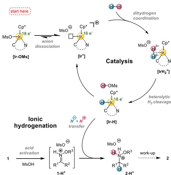
**Scheme 7.** Suggested reaction mechanism of the ionic iridium-catalyzed oxime hydrogenation.
