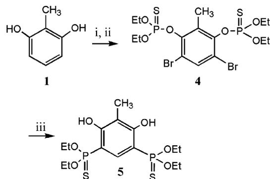
**Scheme 4** Synthesis of the aryl bis(thiophosphonate) **5** following a double [1,3]-phospho-Fries rearrangement. (i)  $\text{Br}_2$ ,  $\text{CH}_3\text{COOH}$ ; (ii)  $\text{Cl-P(S)(OEt)}_2$  (2.2 equivalents),  $\text{NEt}_3$  (2.4 equivalents), DMAP (10 mol%), THF, 20 °C; (iii) *n*-BuLi (2.4 equivalents), THF,  $-78$  °C then water.
