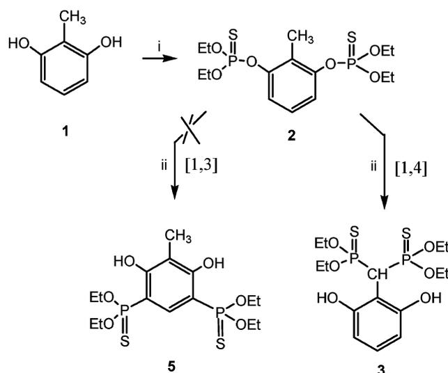
**Scheme 2** Synthesis of *O,O,O,O*-tetraethyl(2,6-dihydroxyphenyl)-methylene-dithiophosphoante **3**: (i) Cl-P(S)(OEt)<sub>2</sub> (2.2 equivalents), NEt<sub>3</sub> (2.4 equivalents), DMAP (10 mol%), THF, 20 °C; (ii) *t*-BuLi, THF,  $-78$  °C then water.
