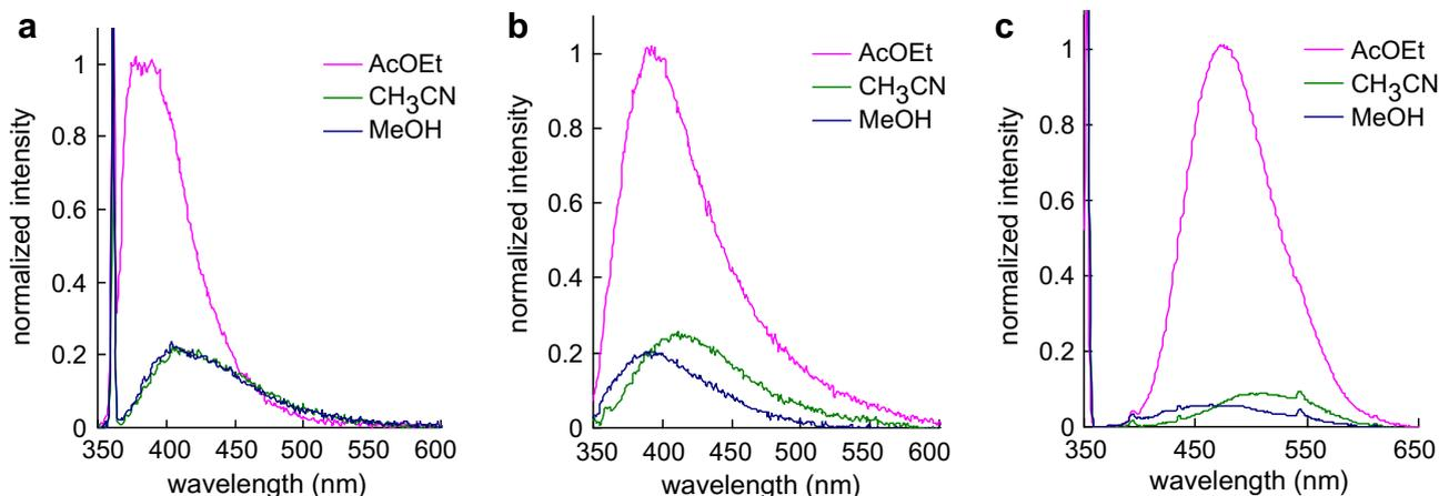
**Figure 2.** Fluorescence spectra of **4a** (a), **4b** (b) and **4c** (c) in various solvent (each 10 μM conc.). Excitation wavelength was 355 nm (a), 345 nm (b), and 350 nm (c).
