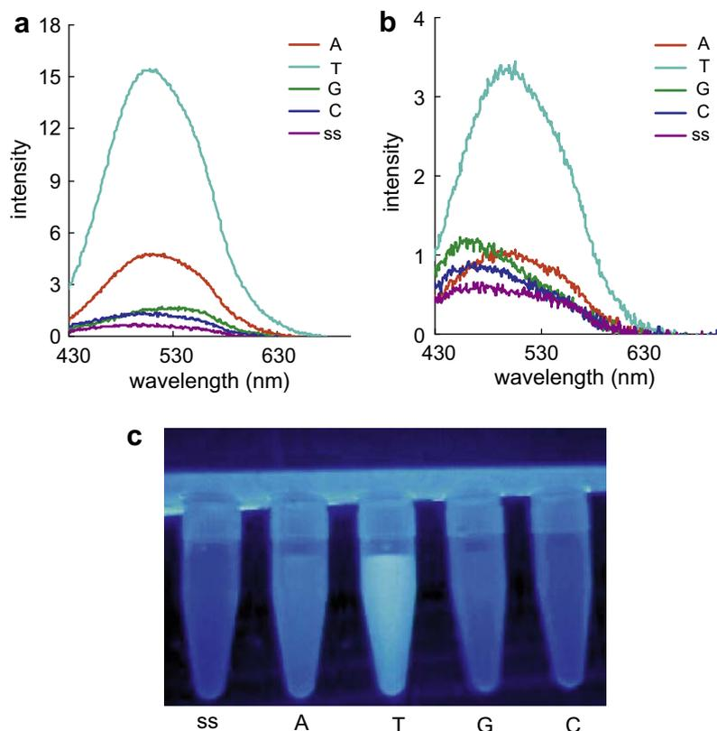
**Figure 3.** Fluorescence spectra of ODN **1** (a) and ODN **2** (b) together with those of the duplexes formed by hybridization with ODN **3** and **4** (N = A, T, G, C), respectively (2.5  $\mu\text{M}$  ODNs, 50 mM sodium phosphate, 0.1 M sodium chloride, pH 7.0, rt). (c) Fluorescence image of ODN **1** (ss) and the duplexes formed with ODN **3** (N = A, T, G, C) under illumination with transilluminator (365 nm). 'ss' denotes single stranded ODN.
