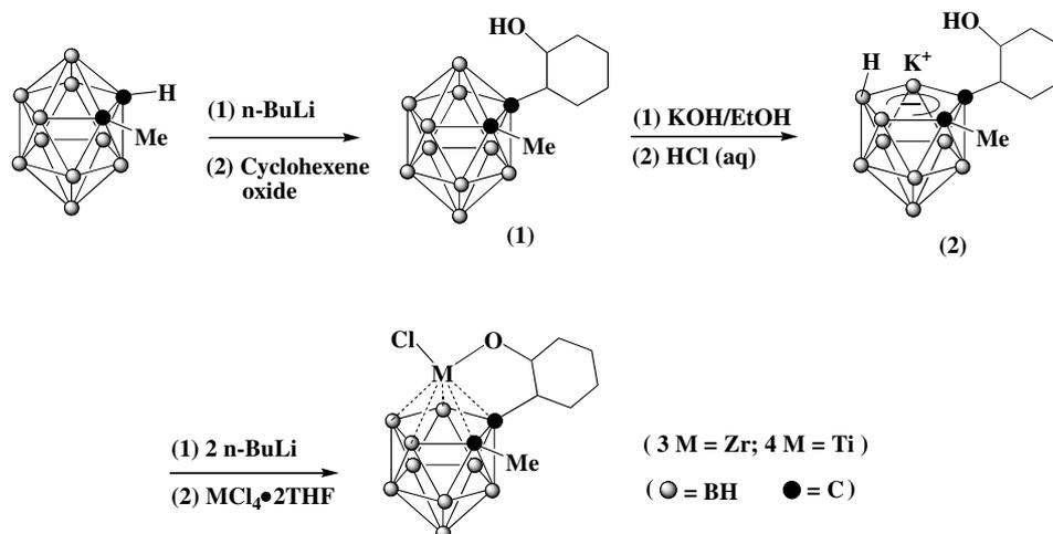
Scheme 1. Synthesis of constrained-geometry Group 4 metallocarboranes.
