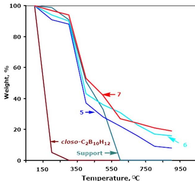
Fig. 2. TGA curves of Merrifield's peptide resin (support), *closo*- $\text{C}_2\text{B}_{10}\text{H}_{12}$ , 5, 6 and 7.
