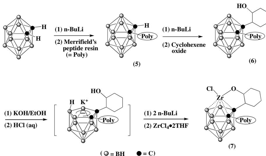
Scheme 2. Synthesis of Merrifield's peptide resin-supported constrained-geometry zirconacarborane.
