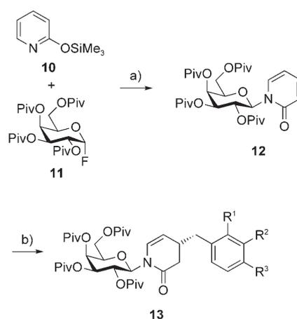
**Scheme 3.** Regio- and diastereoselective synthesis of **13**: a) 1,2-dichloroethane,  $70^\circ\text{C}$ ,  $\text{TiCl}_4$ , 2 h, 99%; b) TIPSOTf, DCM, room temperature, 1 h, then 2,6-lutidine,  $\text{RMgX}$ ,  $20^\circ\text{C}$ , 2 h (Table 1).
