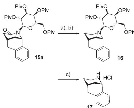
**Scheme 5.** Synthesis of 7,8-benzomorphan: a) Lawesson's reagent (0.5 equiv), toluene, 110 °C, 1.5 h, 83%; b) Raney Ni, H<sub>2</sub>, *i*PrOH, 70 °C, 2 h, 74%; c) 2 N HCl in methanol, 20 °C, 24 h, 96%.
