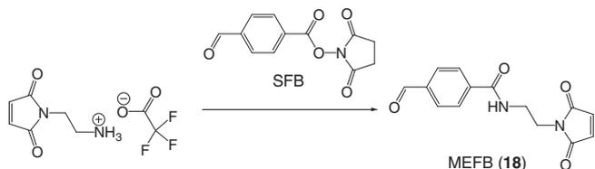
**Scheme 6.** Schematic depiction of the synthesis of the crosslinker MEFB (**18**). Reagents and conditions: phosphate buffer, MeCN, pH 7.2, 60 min, 55% yield.
