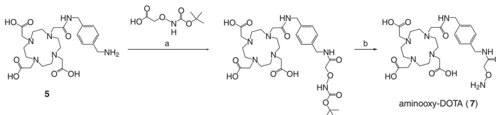
**Scheme 4.** Synthesis route for aminoxy-DOTA (**7**). Reagents and conditions: (a) HBTU, DIPEA, DMF, 30 min (not isolated); (b) TFA, TIS, 15 min, overall yield: 28% yield.
