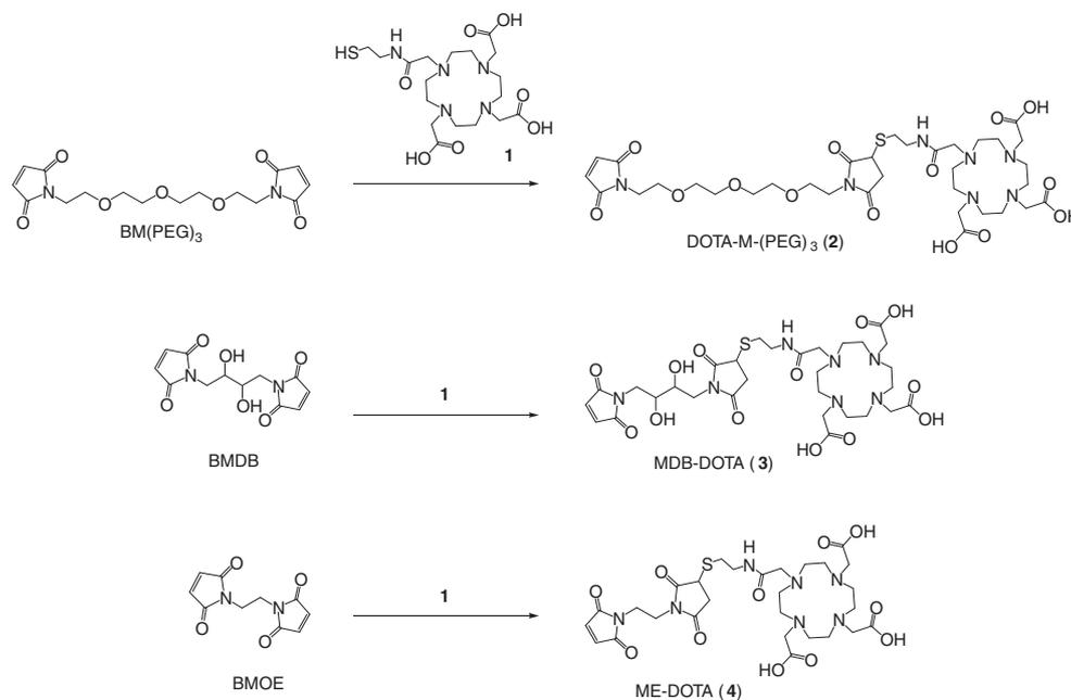
**Scheme 1.** Reaction pathway for the syntheses of the DOTA-maleimides DOTA-M-(PEG)<sub>3</sub> (**2**), MDB-DOTA (**3**), and ME-DOTA (**4**) obtained by reacting BM(PEG)<sub>3</sub>, BMDB, and BMOE with thiol-DOTA (**1**). Reagents and conditions: phosphate buffer, pH 7.2, 5 min, 57%, 40%, and 48% yields.
