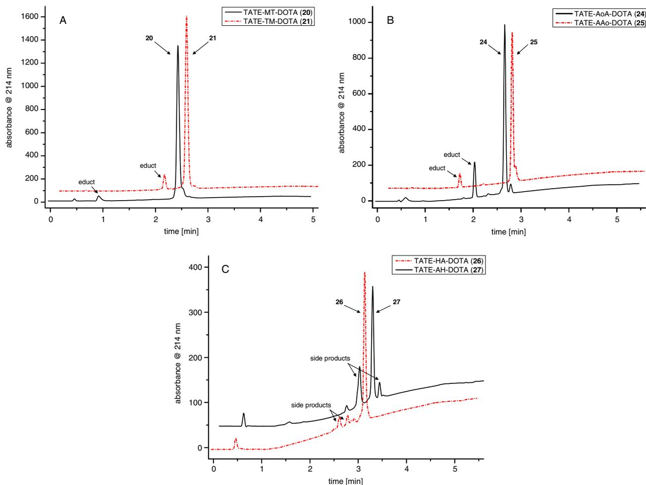
**Figure 2.** Analytical HPLC-chromatograms of conjugation reaction mixtures of (A) **1** with **13** (solid line) and **14** with **2** (dashed line) after 5 min reaction time; (B) **6** with **15** (solid line) and **7** with **19** (dashed line) after 5 min reaction time; (C) **9** with **17** (solid line) and **10** with **16** (dashed line) after 60 min reaction time.
