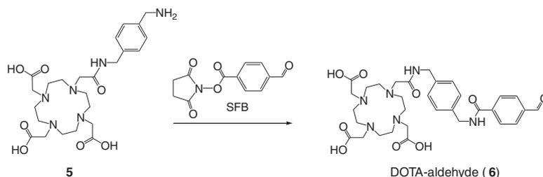
**Scheme 3.** Reaction pathway for the synthesis of DOTA-aldehyde (**6**) starting from amino-DOTA (**5**). Reagents and conditions: phosphate buffer, MeCN, pH 7.2, 1 h, 37% yield.
