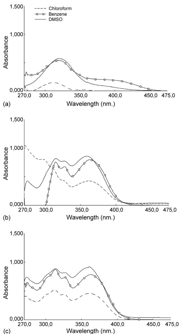
Fig. 1. The UV-vis spectra of compound **6** in (a) acidic, (b) neutral and (c) basic media.
