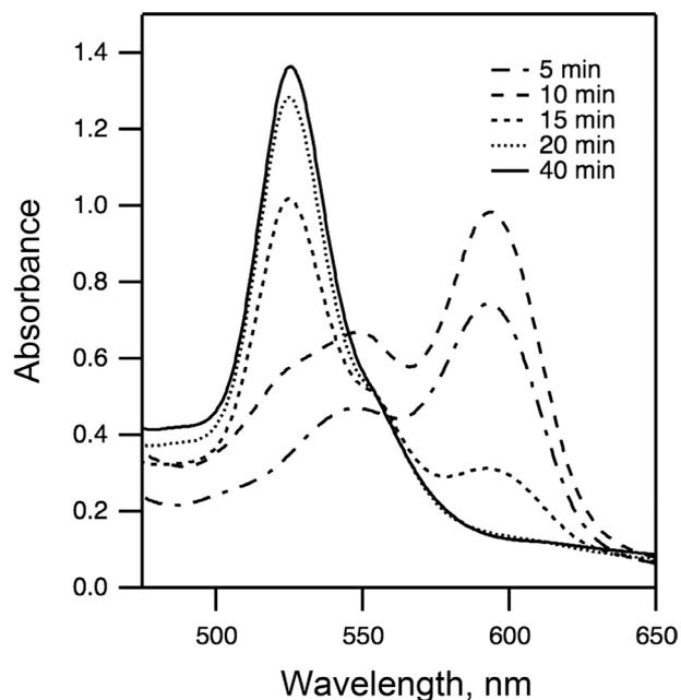
**Fig. 3.** The UV-visible spectra recorded after sampling at the intervals shown, during the microwave heating of **Ni4a** at 240 °C in DMF
