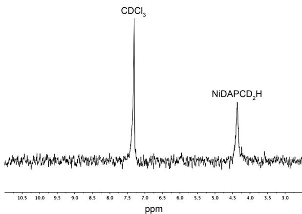
**Fig. 1.** The  $^2\text{H}$  NMR spectrum of NiDAPCD $_2\text{H}$  (**Ni4c**) from the microwave-heated reaction of **Ni4a** in  $d_7$ -DMF at 250 °C
