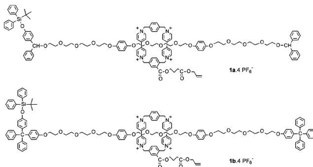
**Figure 1.** Proposed rotaxane monomers for the preparation of oligorotaxanes via the stepwise "polymerization" procedure.
