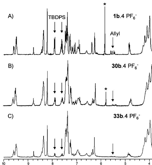
**Figure 2.** <sup>1</sup>H NMR spectra of the tetraphenylmethane-based rotaxanes: (a) monomer **1b**·4PF<sub>6</sub><sup>-</sup>; (b) dimer **30b**·8PF<sub>6</sub><sup>-</sup>; (c) tetramer **33b**·16PF<sub>6</sub><sup>-</sup>. The asterisk marks a signal due to residual solvent.
