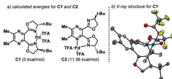
**Figure 1.** a) Energy profile for complexes **C1** and **C2**. b) X-ray structure of **C1**. Ellipsoids set at 50% probability.
