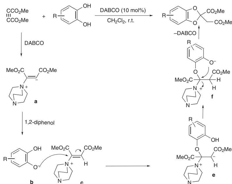
**Scheme 2** Plausible mechanism for the reaction of 1,2-diphenols with DMAD.
