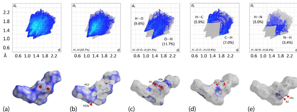
**Fig. 7.** (a) The overall two-dimensional fingerprint plot for **1** as well as those delineated into (b) H...H, (c) H...O/O...H, (d) H...C/C...H and (e) H...N/N...H contacts, with the prominent tips of the fingerprint plot corresponding to the relevant contacts highlighted on the Hirshfeld surface by red cursors.
