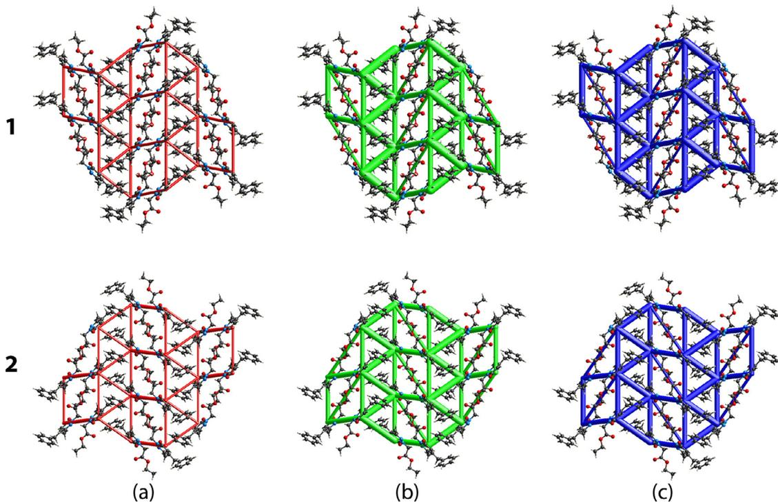
**Fig. 9.** The calculated energy frameworks for **1** and **2** as viewed along the a-axis, showing the (a) electrostatic force (red cylinders), (b) dispersion force (green) and (c) total energy (blue) diagrams. The cylindrical radius is proportional to the relative strength of the corresponding energies and they were adjusted to the same scale factor of 150 with a cut-off value of 1.9 kcal/mol within a  $2 \times 2 \times 1$  unit-cells.
