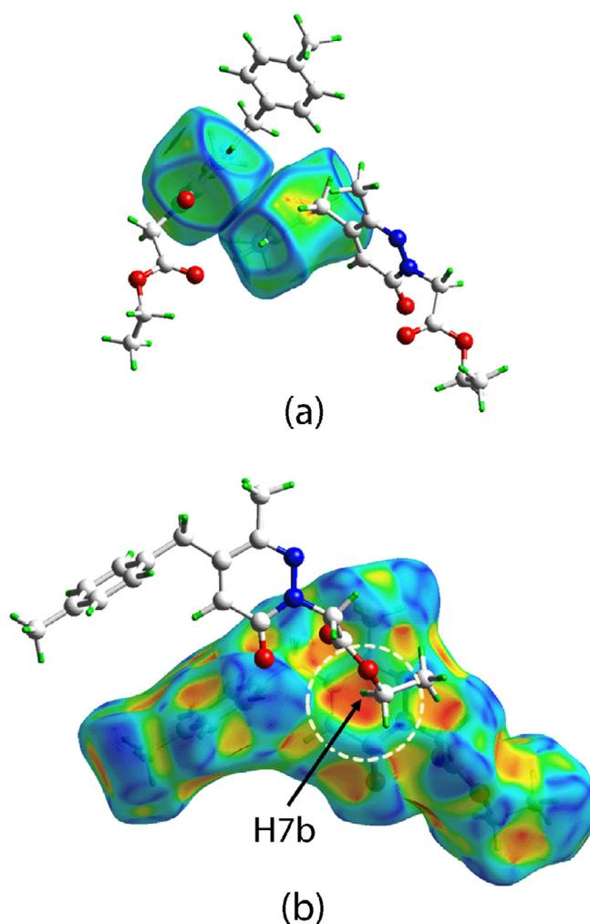
**Fig. 6.** (a) The Hirshfeld surface mapped with curvedness (property range:  $-4.0$  to  $+0.4$  arbitrary units) for  $\pi(\text{N1-C4})\cdots\pi(\text{C11-C16})$  and (b) Hirshfeld surface mapped with the shape index property (range:  $-1.0$  to  $+1.0$  arbitrary units) for the pyridaziny ring (highlighted by the circle) interacting with the methylene-H7b atom.
