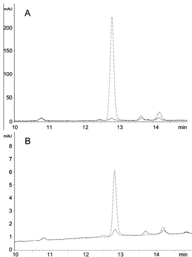
**Figure 2.** Overlay of HPLC traces of Con8 cells incubated with **2** under normoxic (---) and hypoxic (—) conditions: (A) culture supernatant, (B) cell lysate. Equivalent amounts of lysate or supernatant were sampled and after sample preparation were analyzed by HPLC. Y-axis represents absorbance units (mAU) at 370 nm; x-axis indicates time of HPLC run.  $R_t$  (**2**) = 12.9 min. Note difference in vertical scale between panels A and B.
