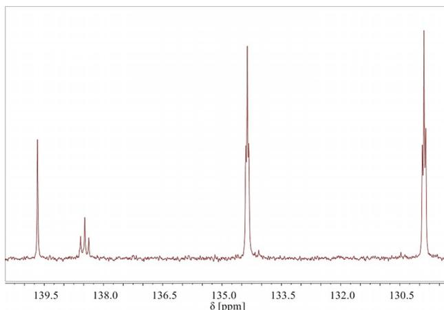
**Figure 1.**  $^{13}\text{C}\{^1\text{H}\}$  NMR spectrum of **5** in  $[\text{D}_8]\text{THF}$  depicting the AA'X coupling pattern of the aryl carbon atoms.
