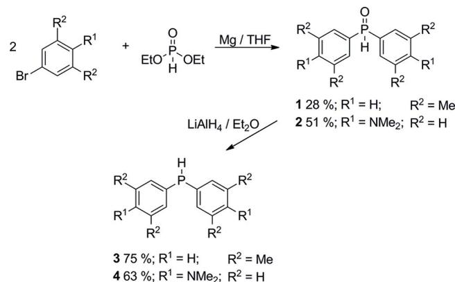
**Scheme 2.** Synthesis of secondary phosphanes of the type  $\text{HP(R)Aryl}$ .
