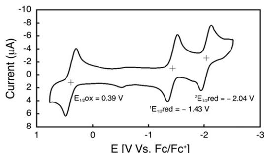
**Fig. 3.** Cyclic voltammogram of **2a** in THF containing tetrabutylammonium perchlorate as supporting electrolyte (vs Fc/Fc<sup>+</sup>).
