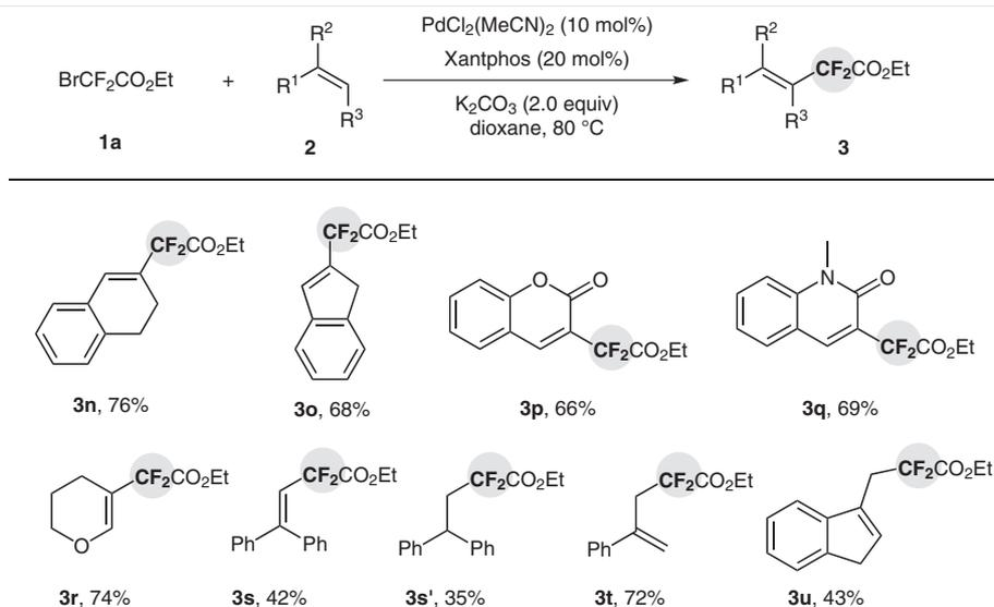
**Scheme 2** Pd-catalyzed ethoxycarbonyldifluoromethylation of branched alkenes with ethyl bromodifluoroacetate (**1a**). *Reagents and conditions* (unless otherwise specified): **1a** (0.6 mmol, 2.0 equiv), **2** (0.3 mmol, 1.0 equiv), 1,4-dioxane (2 mL), 24 h. All reported yields are isolated yields.
