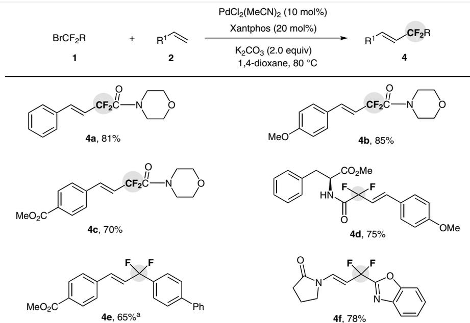
**Scheme 3** Pd-catalyzed Heck-type reaction of functionalized difluoromethyl bromides with alkenes. *Reagents and conditions* (unless otherwise specified): **1** (0.6 mmol, 2.0 equiv), **2** (0.3 mmol, 1.0 equiv), 1,4-dioxane (2 mL), 24 h. All reported yields are isolated yields. <sup>a</sup> Molecular sieves (3 Å) were used.
