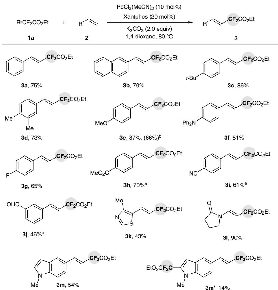
**Scheme 1** Pd-catalyzed ethoxycarbonyldifluoromethylation of linear alkenes with ethyl bromodifluoroacetate (**1a**). *Reagents and conditions* (unless otherwise specified): **1a** (0.6 mmol, 2.0 equiv), **2** (0.3 mmol, 1.0 equiv), 1,4-dioxane (2 mL), 24 h. All reported yields are isolated yields. <sup>a</sup> Molecular sieves (3 Å) were used. <sup>b</sup> The reaction was carried out on a 1-gram-scale.
