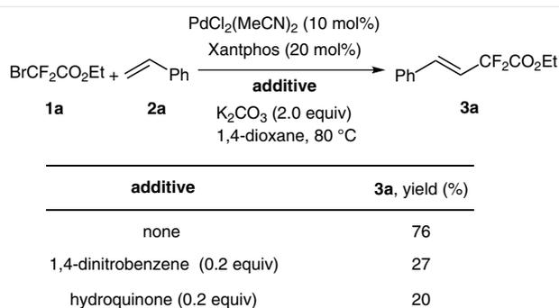
**Scheme 5** Inhibition experiments for Pd-catalyzed cross-coupling of **1a** with **2a**
