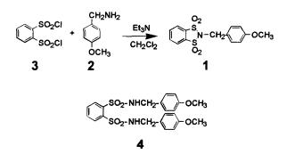
Compound 1 was a stable product with mp. 146-7 °C. Formation of the *o*-benzenedisulfonamide 4 was suppressed by the slow addition of the amine to a refluxing solution of 3 in dichloromethane.
