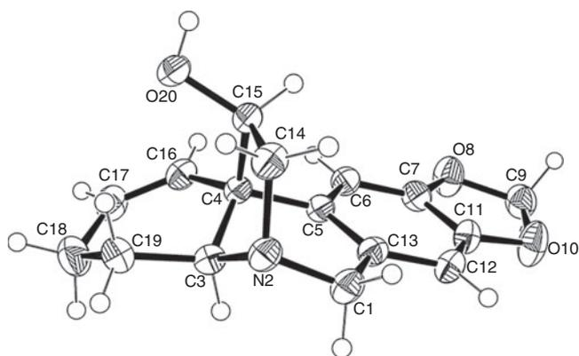
**Fig. 4.** ORTEP diagram derived from the single-crystal X-ray analysis of ( $\pm$ )-haemultine [( $\pm$ )-**1**]. Thermal ellipsoids are drawn at the 50% probability level. H atoms are shown as spheres of arbitrary radius.
