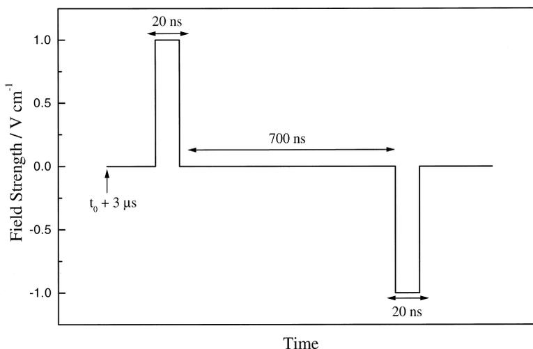
Fig. 1. Schematic of a typical field ionization pulse used in a FSSFI ZEKE experiment. The pulse is applied 3  $\mu$ s after photoexcitation ( $t_0$ ).
