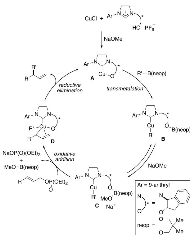
**Scheme 1.** A possible catalytic cycle for the copper-catalyzed allylic substitution of allyl phosphates.
