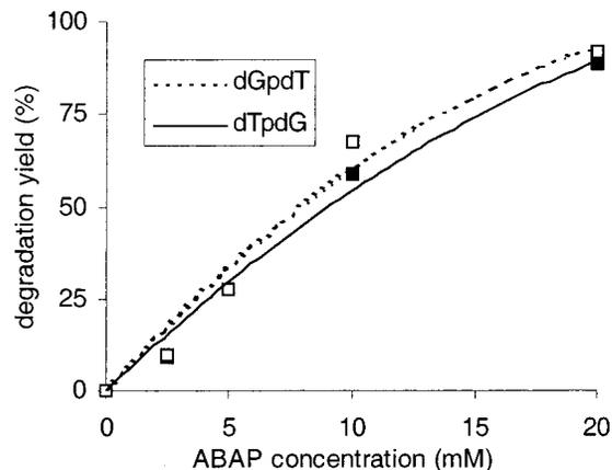
**Figure 3.** Degradation of dGpdT and dTpdG upon incubation with large concentrations of ABAP in aerated aqueous solution at 37 °C. The amount of dinucleoside monophosphate was inferred from HPLC-UV analysis. Dinucleoside monophosphates were solubilized at 1 mM concentration in 10 mM, pH 7, phosphate buffer. The reported values represent the average of two independent determinations.
