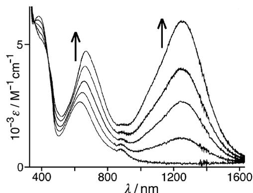
Fig. 3 Electronic spectra recorded during oxidation of **1** to [1]<sup>+</sup> in an OTTLE cell (CH<sub>2</sub>Cl<sub>2</sub>, 243 K).
