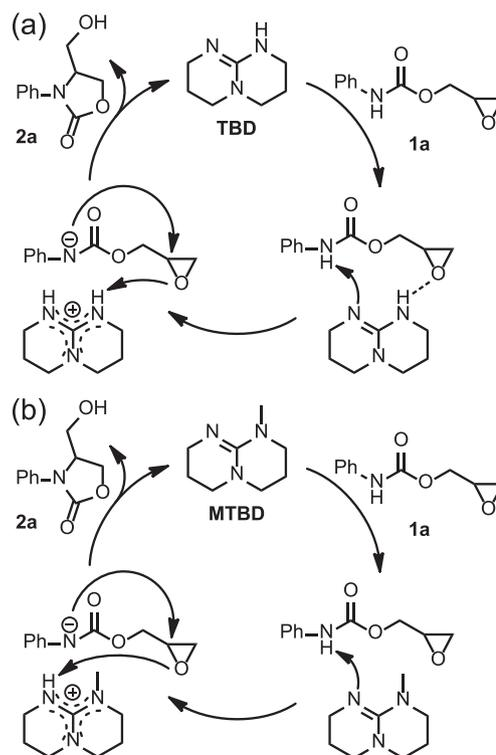
**Scheme 1.** Speculated mechanism of the intramolecular cyclization from **1a** to **2a** catalyzed with (a) TBD and (b) MTBD.
