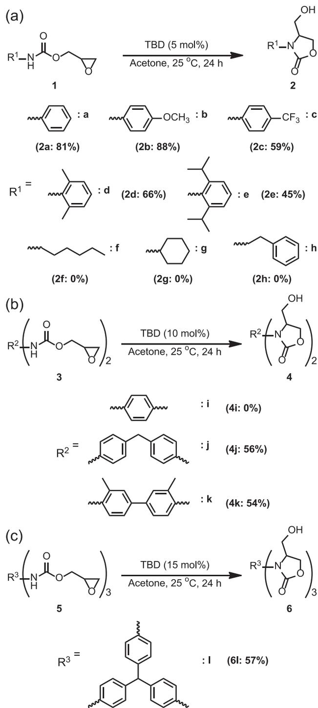
**Scheme 2.** Synthesis of 4-hydroxymethyl 2-oxazolidinone derivatives with TBD in acetone at 25 °C for 24 h from, (a) glycidyl carbamates having various functional groups, (b) bifunctional glycidyl carbamates having aromatic groups, and (c) trifunctional glycidyl carbamate.
