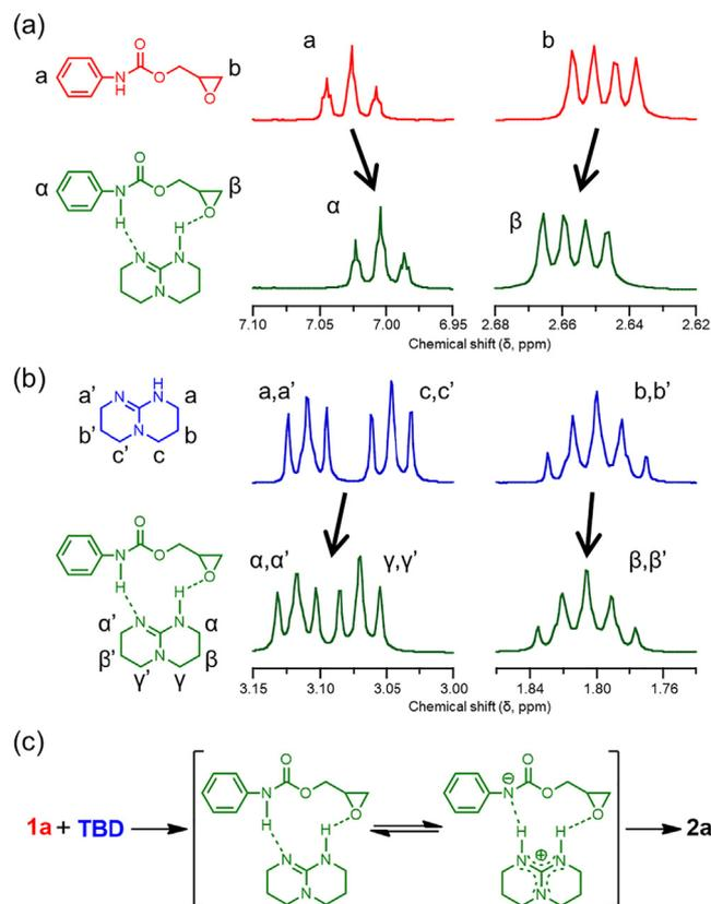
**Fig. 2.** <sup>1</sup>H NMR spectra of stoichiometric mixture of **1a** and TBD. (a) Chemical shift of the protons assigned to phenyl group and epoxy ring. (b) Chemical shift of the protons assigned to TBD. (c) Proposed structure of the intermediate prepared with **1a** and TBD.
